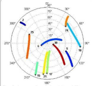
**Fig. 7** Skyplot corresponding to the Seewinkel network. PRN6 is taken as the reference satellite for the computation of the DD
