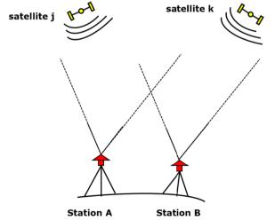
**Fig. 1** Geometry of the relative positioning and DD; the rays are almost parallel at the stations A and B due to the great distance to the satellites of 20,000 km ( $\sim$  0.01° difference for a 1 km station separation)
