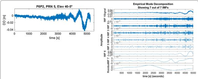
Fig. 8 Left: DD residuals in [m] for PRN5, baseline P0P2. Right: the corresponding EMD decomposition using seven modes, pchip and a threshold of 1e<sup>-6</sup>
