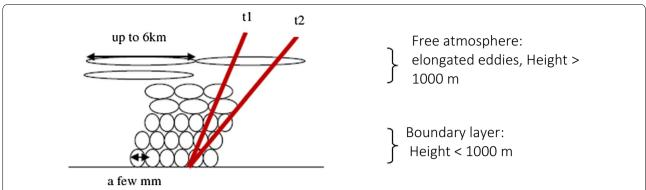
**Fig. 4** GNSS signal path through the turbulent troposphere using the concept of isotropic eddies in the boundary layer and anisotropic two-dimensional structure in the free atmosphere. *t*1 and *t*2 are two epochs of measurements. The figure is adapted from Kermarrec and Schön (2014)
